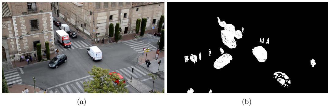
Figure 2.11: Example of blob merge due to partial occlusions and blob split due to a tree, after applying background subtraction. (a) Original image. (b) Foreground mask.
