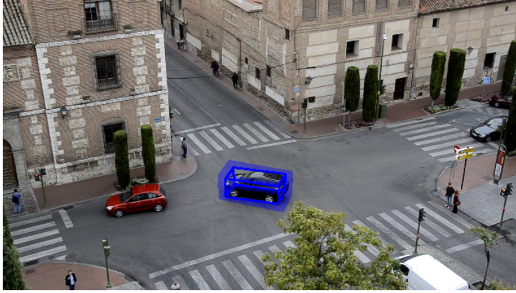
Figure 3.38: Projected vehicle volume under maximum VP range variations.
