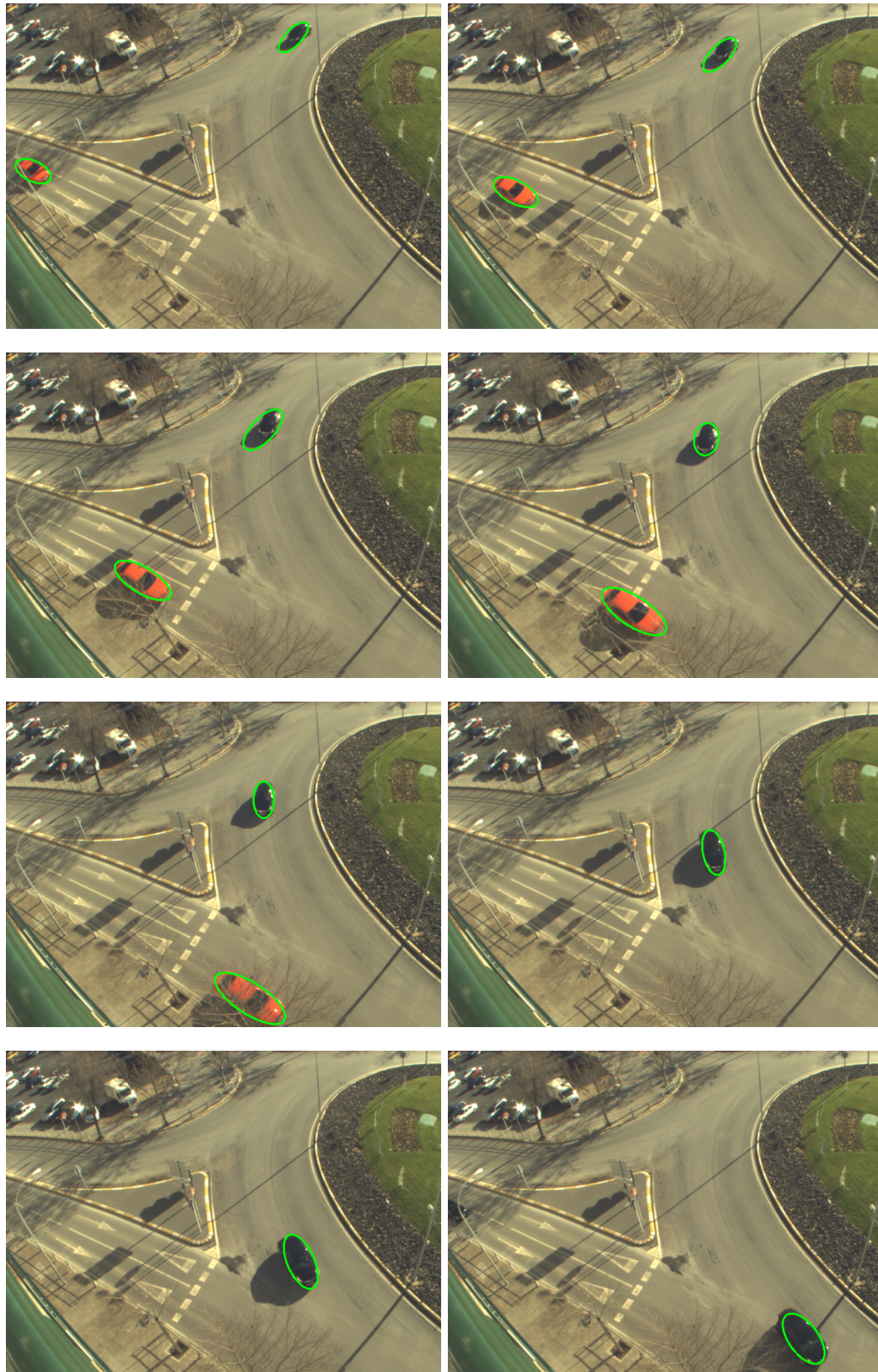
Figure 4.39: Graphic results of video 6. Samples in sunny conditions with representative shadows.
