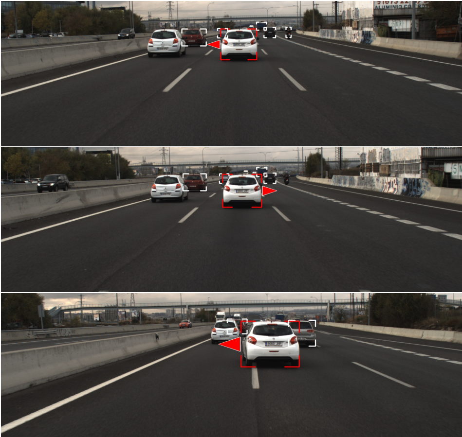
Figure 6.13: Example of lane-change maneuver detection V.
