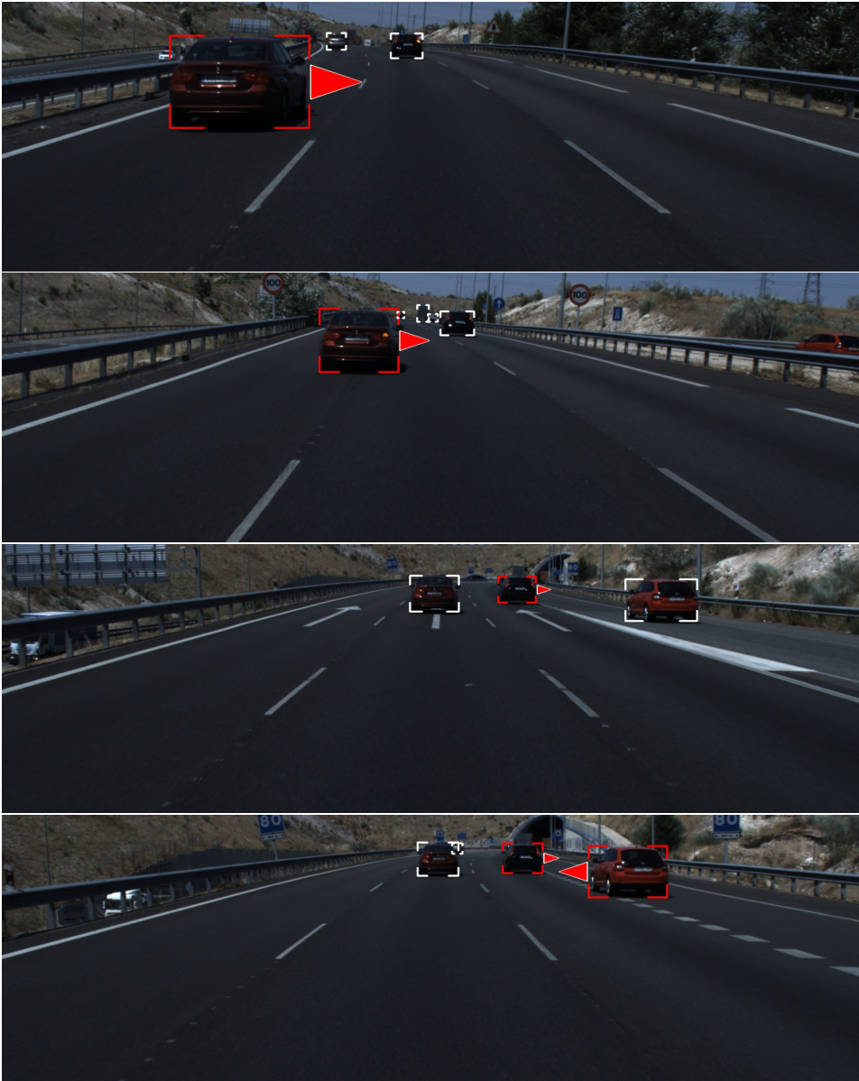
Figure 6.11: Example of lane-change maneuver detection III.
