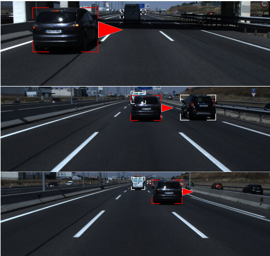
Figure 6.10: Example of lane-change maneuver detection II.
