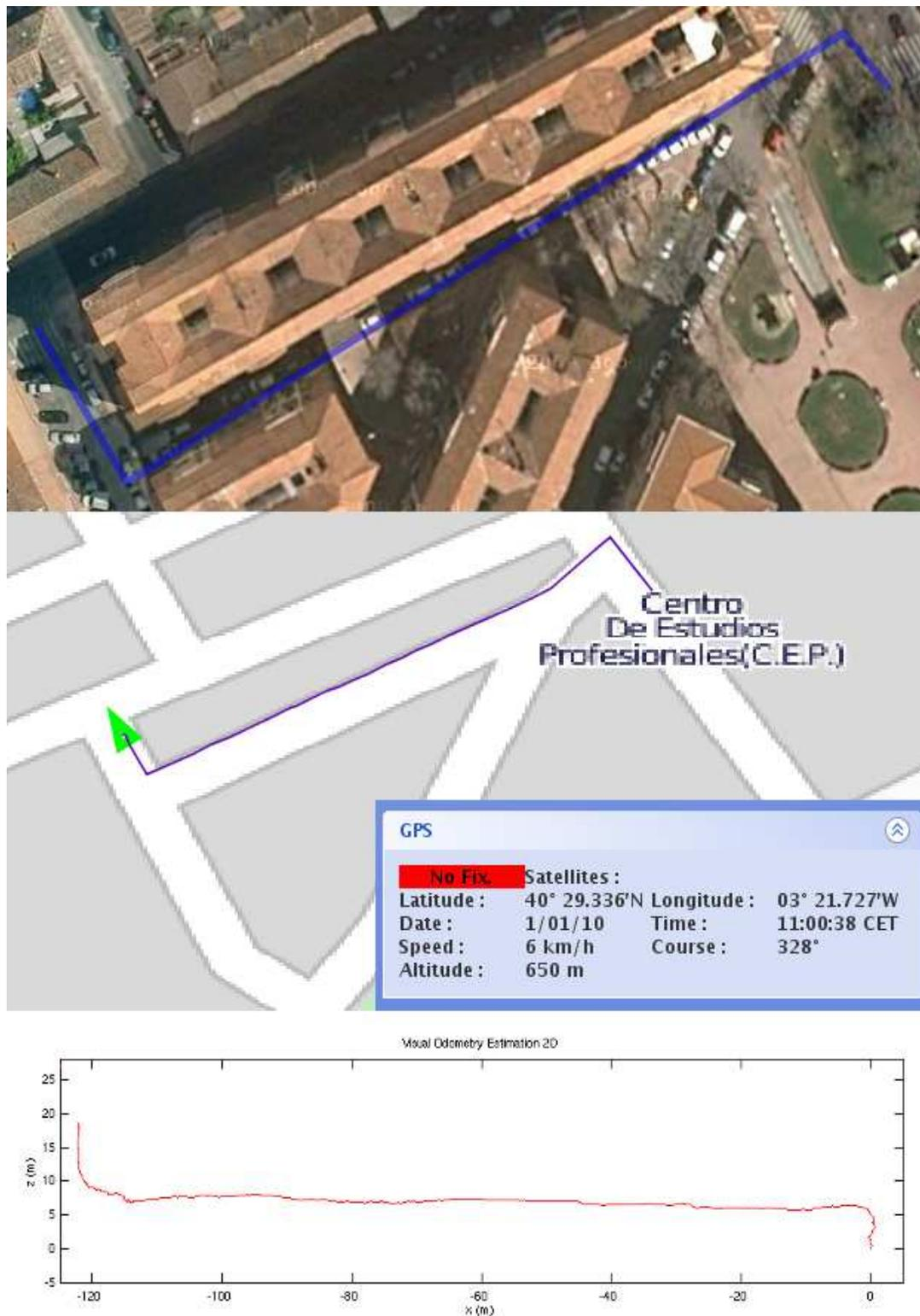
Figure 5.12: On top the vehicle real trajectory displayed in google maps. In the middle the vehicle motion trajectory in the OSM map and the GPS information as shown to the user. Below the raw visual odometry information used to get the vehicle position in the map during the GPS outage
