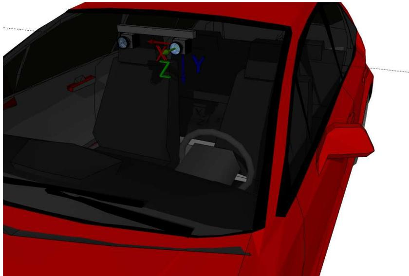
Figure 4.8: Camera coordinate system
