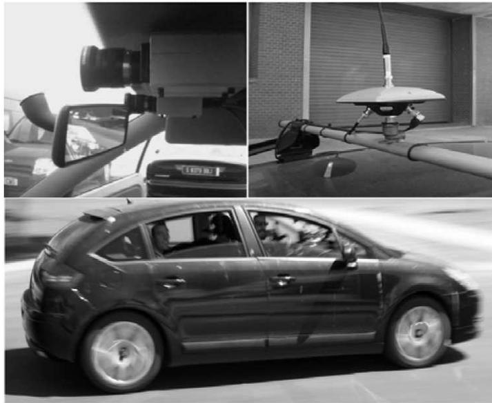
Figure 4.11: (Top left) Stereo cameras. (Top right) RTK-GPS. (Bottom) Experimental Vehicle
