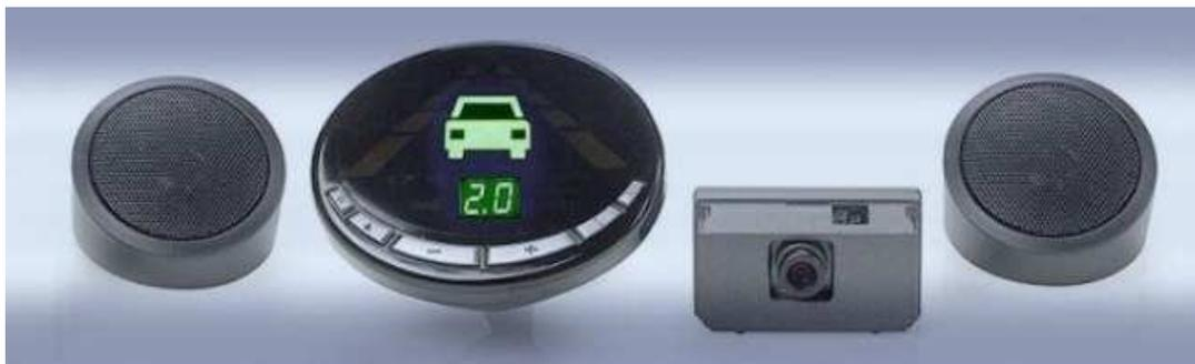
Figure 1.1: Mobileye AWS-4000 camera based safety solution. It performs forward collision warning, lane departure warning and headway monitoring and warning with a single camera.
