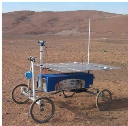
(a) Solar powered robot used in the experiments
