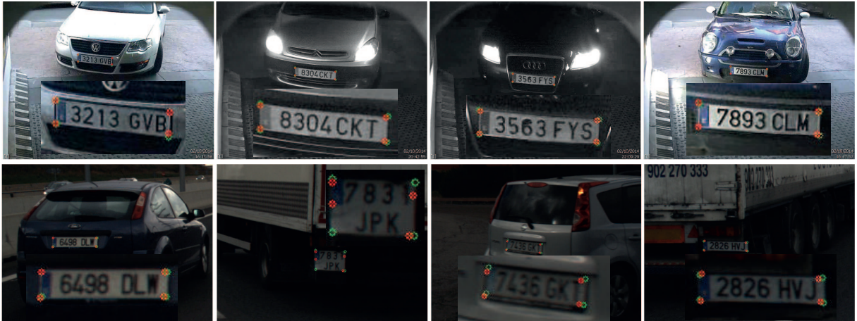
Figure A.4: Examples of license plate corners detection on the validation set (top row) and on the test set (bottom row). Green circles are the ground truth, red circles are the predictions. License plate area has been zoomed to ease visualisation.
