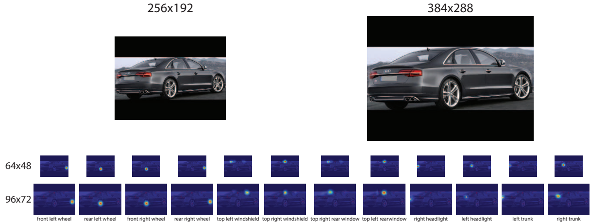
Figure 5.1: Visual comparison of the input size and output heatmaps for ResNet50 256x192 and ResNet152 384x288 models. On top the input images, in the middle the ResNet50 256x192 output heatmaps and on the bottom the ResNet152 384x288 output heatmaps.
