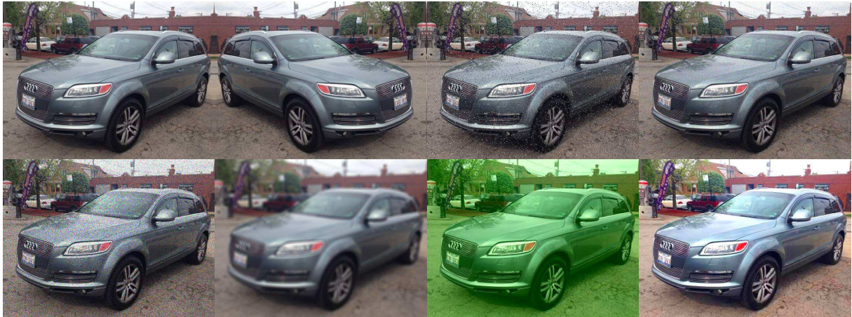
Figure 4.3: Visual examples of the different data augmentation operations. On top, from left to right, no data augmentation, horizontal flip, salt-and-pepper noise and poisson noise. On bottom, from left to right, speckle noise, blurring, colour casting, and colour jittering.
