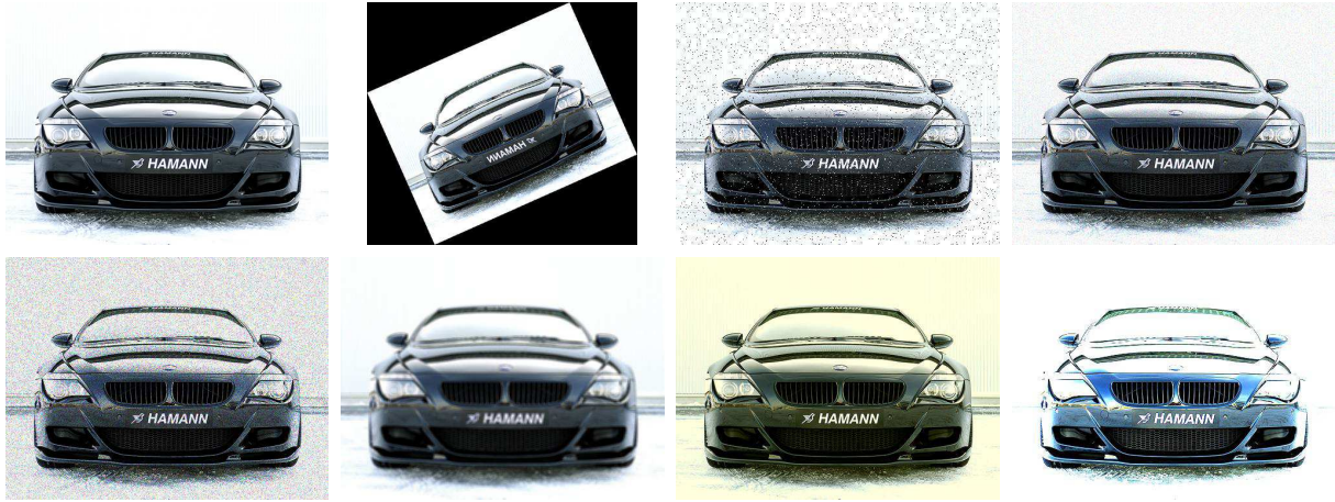
Figure 3.3: Visual examples of the different data augmentation operations. On top, from left to right, no data augmentation, mild data augmentation (with horizontal flip, rotation and scaling), salt-and-pepper noise and poisson noise. On the bottom, from left to right, speckle noise, blurring, colour casting, and colour jittering. The hard data augmentation specific operations have been performed over the original image without the mild data augmentation to ease visualisation.
