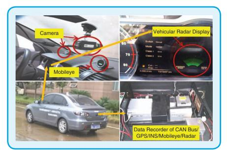
FIG 4 Experimental vehicle and apparatus.
