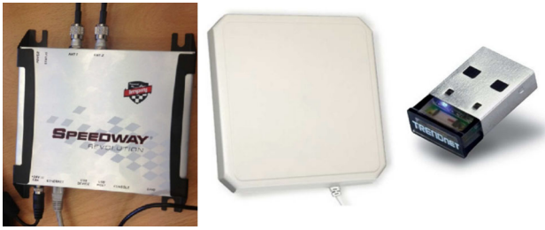
Fig. 6 Left UHF Class 1 Gen 2 RFID Speedway Revolution R220 reader. Middle far field circularly polarized panel antennas within the 865–870 MHz band (Europe frequency allocation). Right Trendnet Class I micro Bluetooth 4.0 USB adapter with BLE protocol (2.4 GHz)
