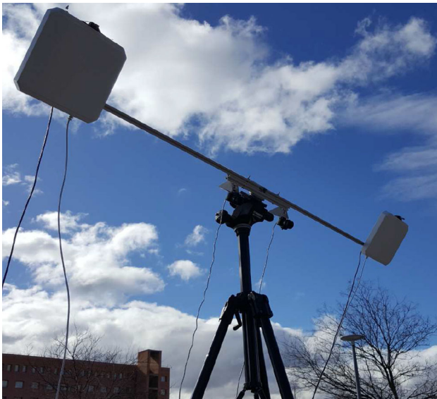
Fig. 7 Sensor setup including stereo cameras (baseline of 30 cm), RFID antennas and BLE adapters (baseline of 3 m)
