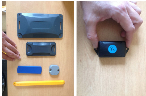
Fig. 5 Left RFID tags (including Onmi-ID Dura 3000). Right BLE beacon from GeLo Inc
