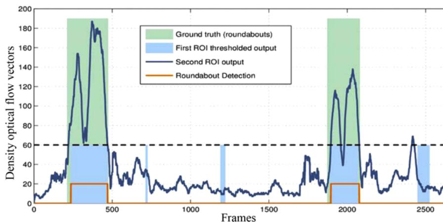
Figure 11. Results of the two optical flow analysis functions.
