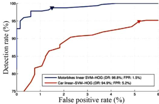
Figure 7. ROC curve of the linear SVM classifier performance.
