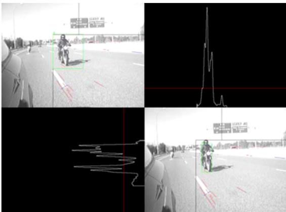
Figure 5. Bounding box fitting using horizontal and vertical edges.
