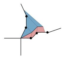
Fig. 4. Implemented curve-to-curve map-matching algorithm. The black points represent the nodes in the map, the thick lines are the road segments, and the dashed line is the estimated trajectory at the interjection exit. In shaded blue and red, the area from the trajectory curve to each one of the intersections exists. The road segment with the smaller area to the trajectory curve will be chosen.
