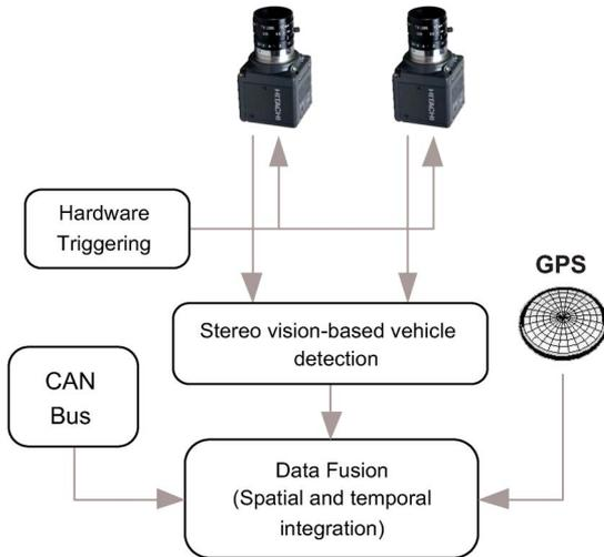
Fig. 2. Global architecture of the xFCD system.
