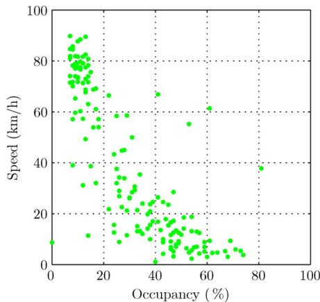
Fig. 17. Route S/O hybrid plane considering the speed values from the xFCD and the occupancy measurements from the magnetic loops.
