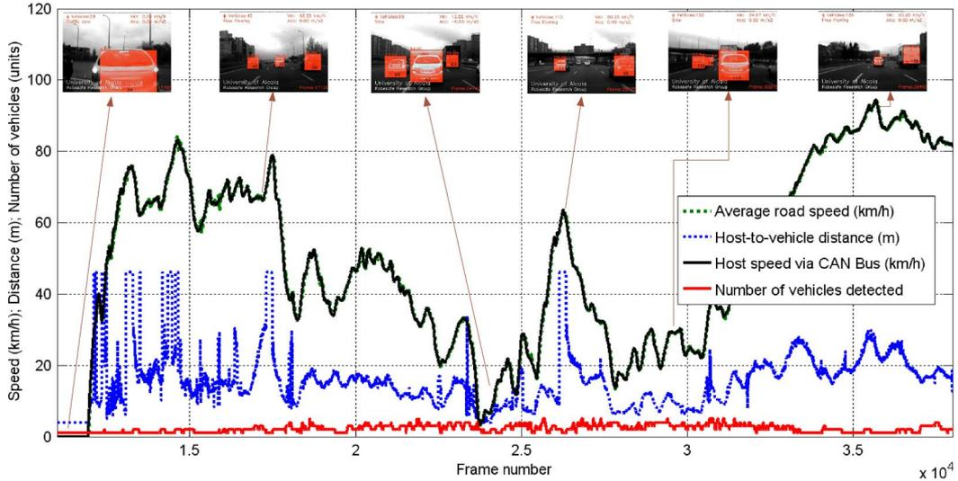
Fig. 12. Vision-based vehicle detection results under daytime, cloudy, and rainy conditions with different levels of traffic congestion, corresponding to 13 min of a sequence.
