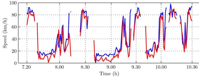
Fig. 14. Speed collected by the (red) vehicle and (blue) fixed loops.
