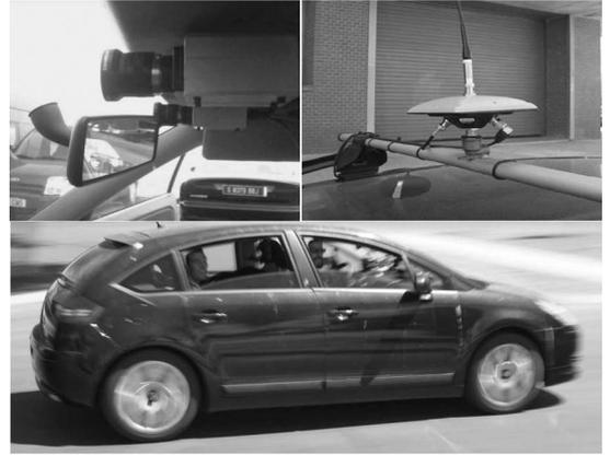
Fig. 1. (Top left) Low-cost stereo vision sensor. (Top right) RTK-DGPS. (Bottom) Experimental vehicle (modified Citroën C4).
