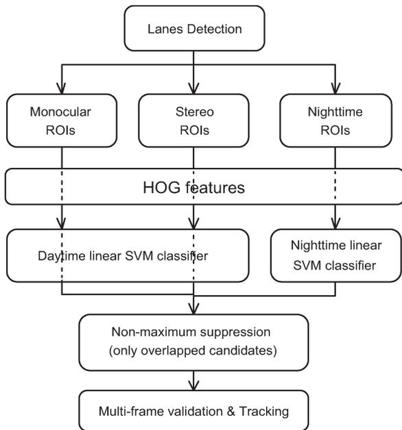
Fig. 3. Global overview of the vision-based vehicle detection algorithm.
