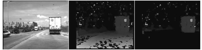
Fig. 4. (Left to right) Original image, dense disparity map, and filtered map (without ground-plane points or points that are very high).
