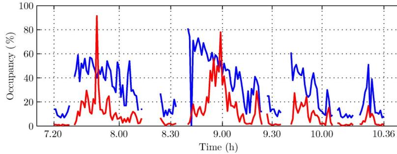
Fig. 15. Occupancy calculated from the number of vehicles (red) counted by the host vehicle and (blue) measured by the magnetic loops.
