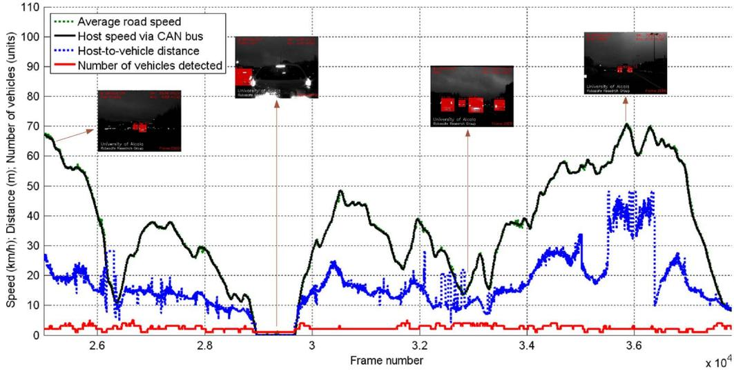
Fig. 13. Vision-based vehicle detection results under nighttime, cloudy, and rainy conditions with different levels of traffic congestion, corresponding to 7 min of a sequence.
