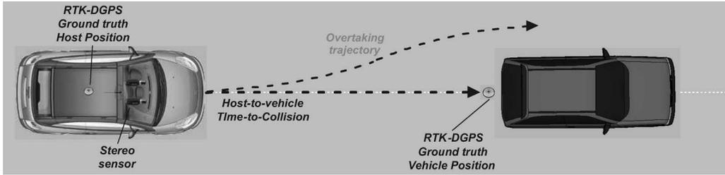
Fig. 7. Scheme of the manual driving experiment.
