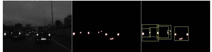
Fig. 5. (Left to right) Original image, individual clusters after adaptive thresholding, and selected ROIs.
