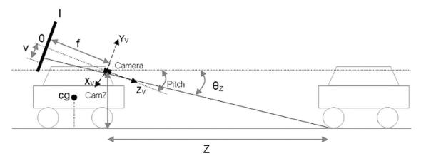
Fig. 5. Vertical road mapping geometry.
