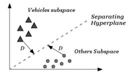
Fig. 11. Vehicle class separation using SVMs.
