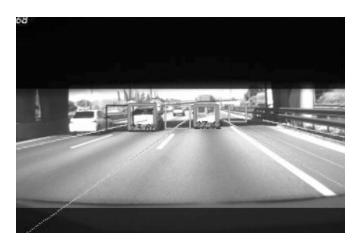
Fig. 22. Example of false vehicle detection.
