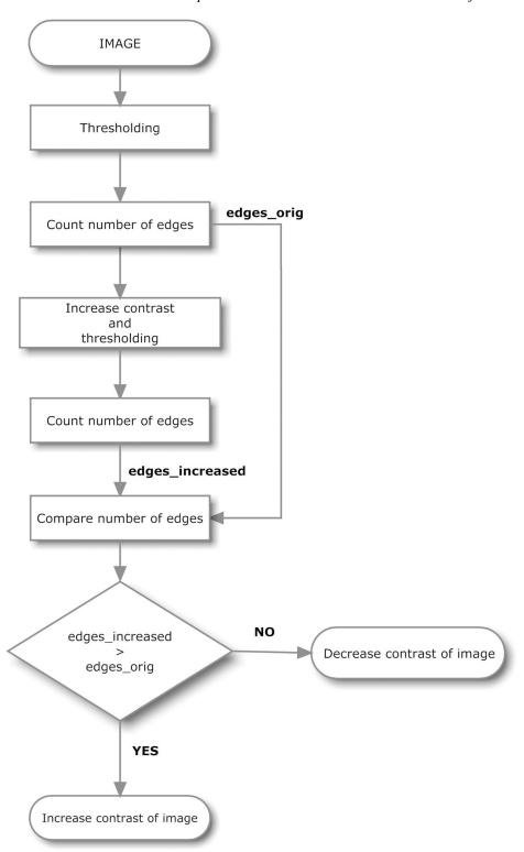
Fig. 3. Block diagram of the adaptive thresholding algorithm.
