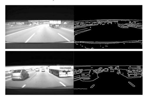
Fig. 2. Edge images after adaptive thresholding.
