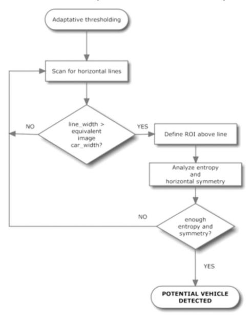
Fig. 6. Block diagram of the vehicle detection mechanism.
