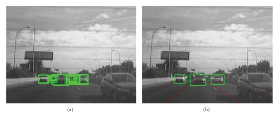
Figure 11: (a) Overlapped candidates. (b) Nonmaximum suppression results.
