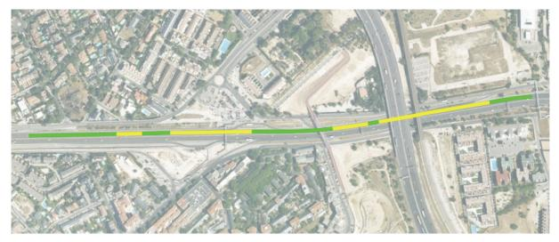
FIGURE 22: GPS trajectory and the corresponding traffic load computed at the central unit (the aerial image has been obtained from Google Earth).
