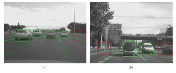
FIGURE 14: Linear SVM with HOG features classification examples: nonvehicle (red) and vehicle (green).
