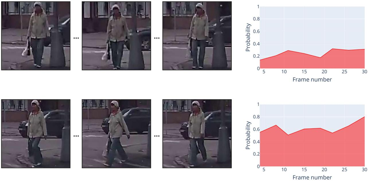
Fig. 4: Two examples in test set. The top one represents a non-crossing sequence and at the bottom, a crossing one. Left graphics show the output crossing probability at eight future time steps between 0 and 1 seconds (0 and 30 frames).
