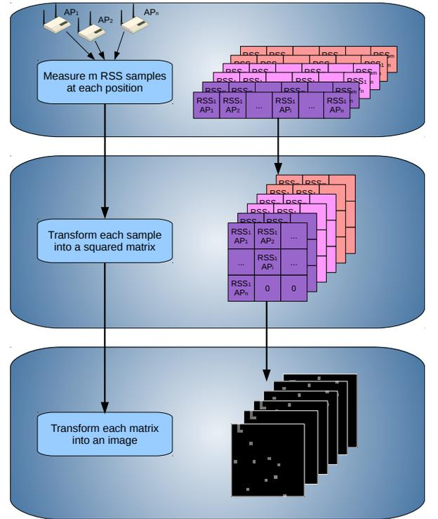
Fig. 6. Collecting and pre-processing data to convert RSS samples into images.
