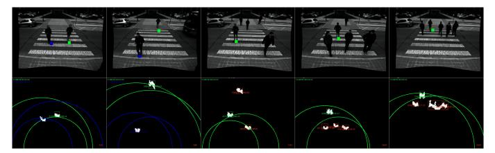
Fig. 4. Upper row: left image with color-coded identification. Lower row: XZ-map (top-view without road points), detected blobs and RSSI circumferences. Each tag is labeled with a different color.
