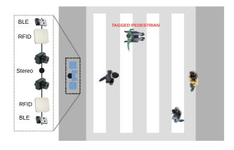
Fig. 1. Pedestrian crossing scenario. Only one (a maximum or two) pedestrians are tagged. The system needs to associate the detected tag with the corresponding pedestrian.
