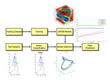
Fig. 1. Pedestrian intention and pose prediction algorithm.
