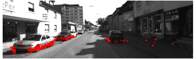
Fig. 3. Points labeled as obstacles using normal vectors
