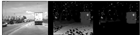
Fig. 4. From left to right: original image, dense disparity map, and filtered map (without ground-plane points or points that are very high).
