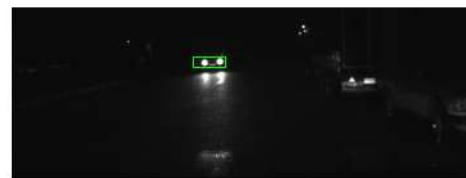
Fig. 11. Detection of an oncoming vehicle
