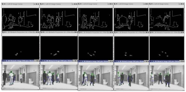
Fig. 6. Results of the classification algorithm in a real situation. Points classified in the obstacles cluster are shown in the images.
