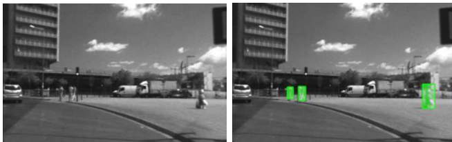
Figure 8: Candidates extraction using texture analysis.
