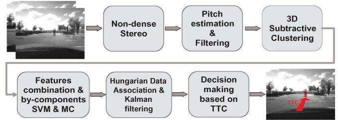
Fig. 4. Overview of the stereo-vision-based pedestrian detection architecture.
