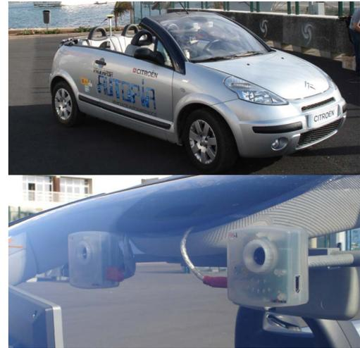
Fig. 1. Experimental vehicle and the onboard stereo sensor.
