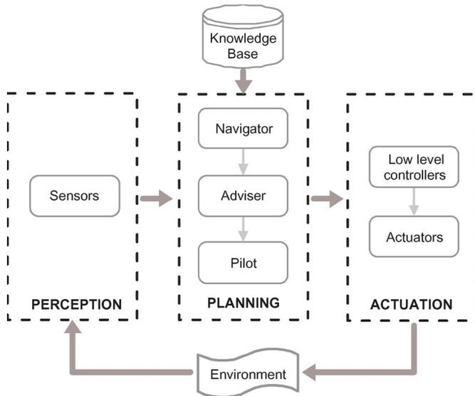
Fig. 3. Stages of the control architecture.
