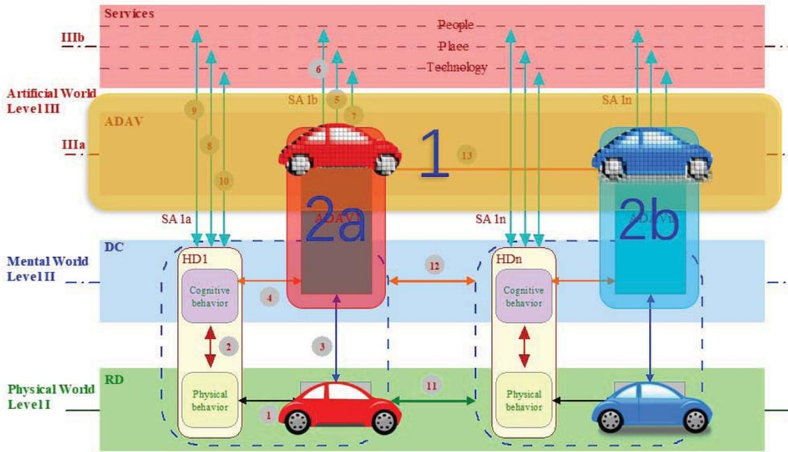
Fig. 4. Parallel driving architecture. RD: real driving; DC: driver cognition; HD: human driver; RV: real vehicle; ADAV: artificial driver and artificial vehicle; SA: situation awareness.
