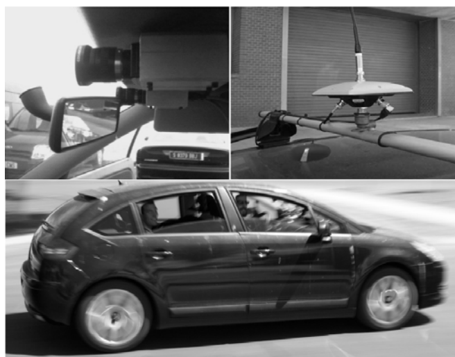
Figure 1. (Top left) Low cost stereo vision sensor. (Top right) RTK-DGPS. (Bottom) Experimental vehicle (modified Citroën C4).
