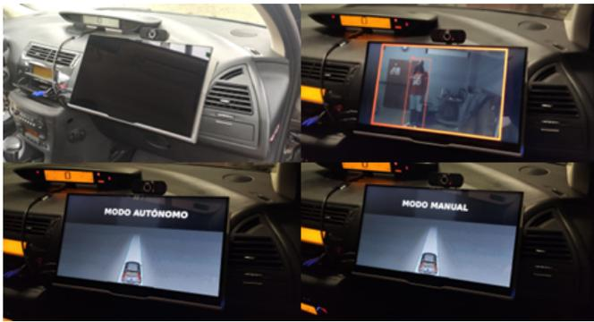
Fig. 6. Internal HMI (iHMI) states: top left *off*, top right *pedestrian detected*, bottom left *autonomous mode*, and bottom right *manual mode*.
