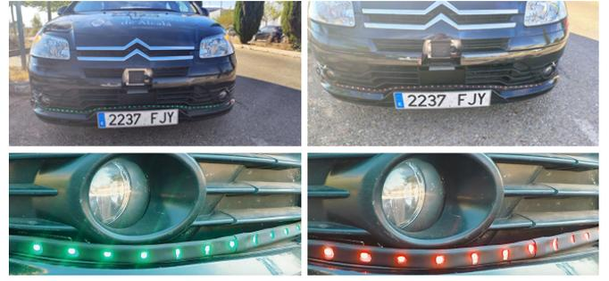
Fig. 5. External HMI (eHMI) - Left *solid green* state and right *solid red* state.
