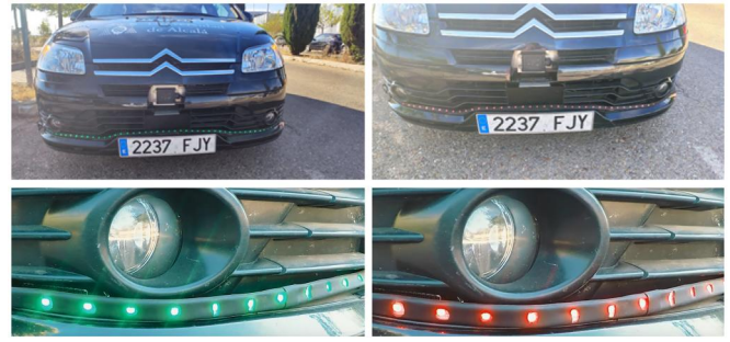
Figure 5. External HMI (eHMI) - left solid green state and right solid red state.
