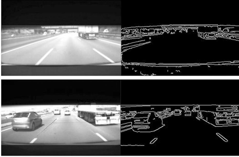
Fig. 2. Edge images after adaptive thresholding.
