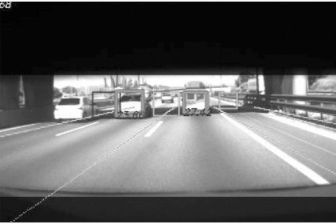
Fig. 22. Example of false vehicle detection.
