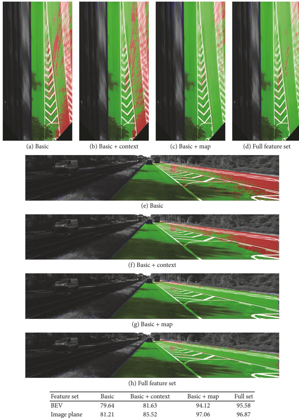
FIGURE 19: Results of unary terms in a specific UMM image. The *map prior* is very important because sometimes the *context feature* does not provide reliable information. The use of the *map prior* in scenarios with multiple marked lanes improves significantly the performance of the basic feature set.
