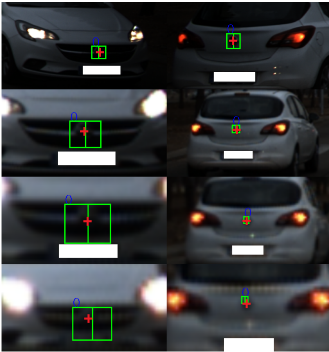
Fig. 5. Vehicle key point tracking. From top to bottom, tracker initialization, and key points after 1, 2 and 3 seconds of tracking using 100 FPS. Left column was tracked in reverse recording order and right column in the forward. 1, 2, 4 and 8 zoom factor have been applied in each row.
