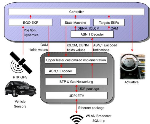
Fig. 3. Flow diagram of the communications system [12].
