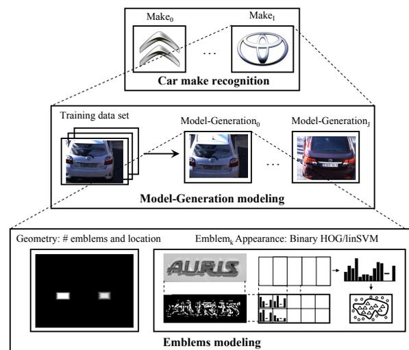
Fig. 2. Overall system layout.
