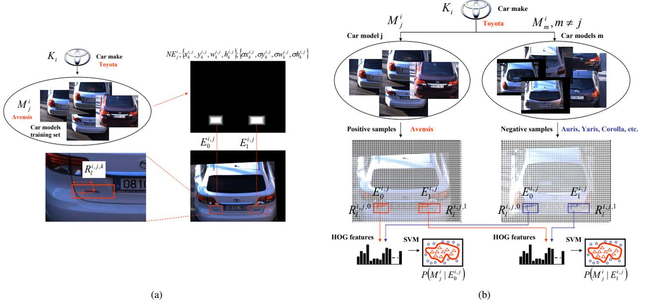
Fig. 4. Learning rear emblems examples: (a) geometry model and (b) appearance model.
