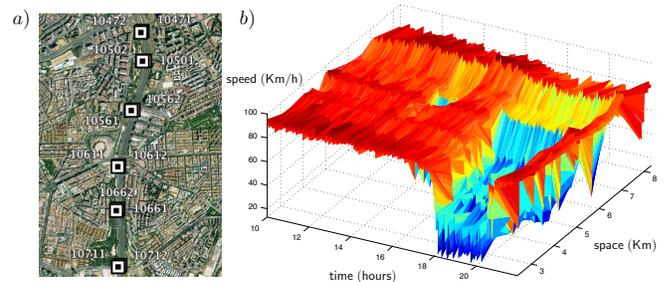
Fig. 1. a) Position of speed sensors in the north-to-south lanes of the M-30 beltway in Madrid, Spain, near the “Puente de Ventas” congestion point. The third digit in each identification number indicates the position of the coil in the beltway in kilometres. b) Spatio-temporal velocity field measured by the aforementioned sensors on November, 8, 2009.
