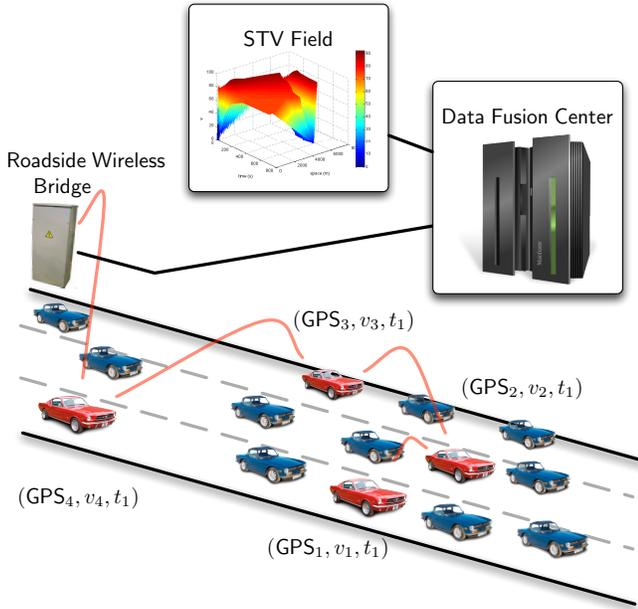
Fig. 2. Outline of the Vehicular Wireless Sensor Network along with the roadside and Data Fusion Centre infrastructure. Blue cars mark the passive cars while red cars mark the sensor vehicles. Red lines indicate the relay channel used to communicate the quasi-synchronous measurements of position ( $GPS_n$ ) and velocity ( $v_n$ ) of different vehicles at different sampling times ( $t_i$ ). This data is provided to the Data Fusion Center for it to calculate the STV field.
