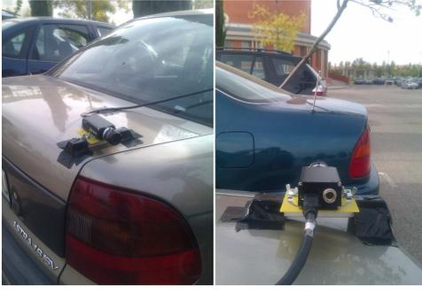
Fig. 2. Camera located at the back-right side of the vehicle.
