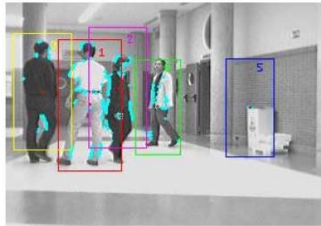
Fig. 4. Results of the position estimator developed in a complex situation, where five objects are being tracked in their movements around the environment.
