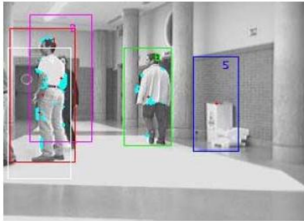
Fig. 4. Results of the position estimator developed in a complex situation, where five objects are being tracked in their movements around the environment.
