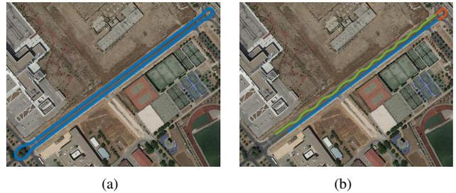
Fig. 7. Experimental environment and trajectories. (a) Trajectory for map creation. (b) Trajectory for localisation tests. In blue, straight line, in red roundabout and in green swerving.
