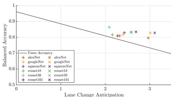
**FIGURE 11. Models performance. Accuracy vs Anticipation. Detection models represented with + symbols and prediction models represented with × symbols. The solid black line represents the average human performance.**
