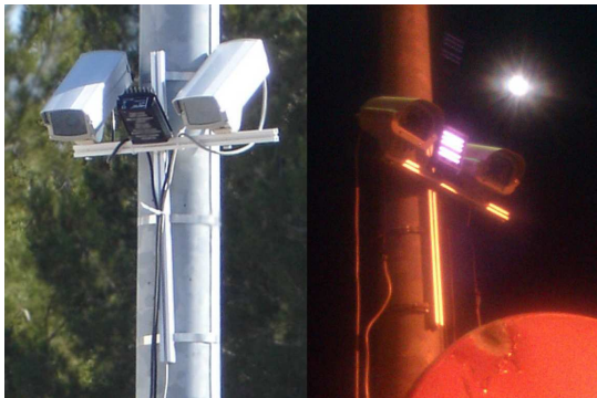
Figure 1: Stereo platform with IR illuminator.
