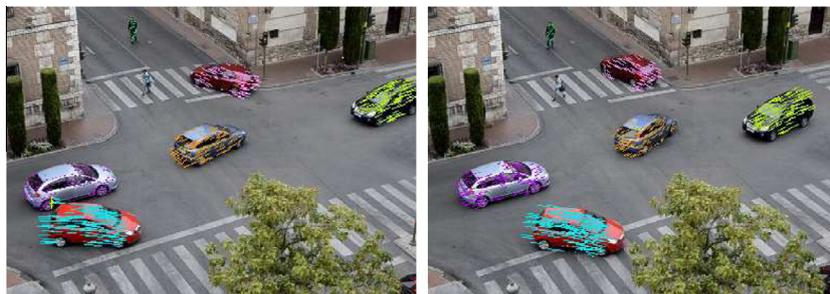
Fig. 14. Examples of feature clustering represented by coloured features.
