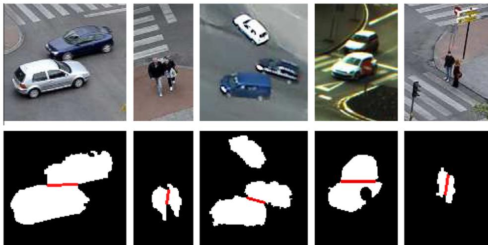
Fig. 13. Examples of occlusion management by the proposed algorithm.
