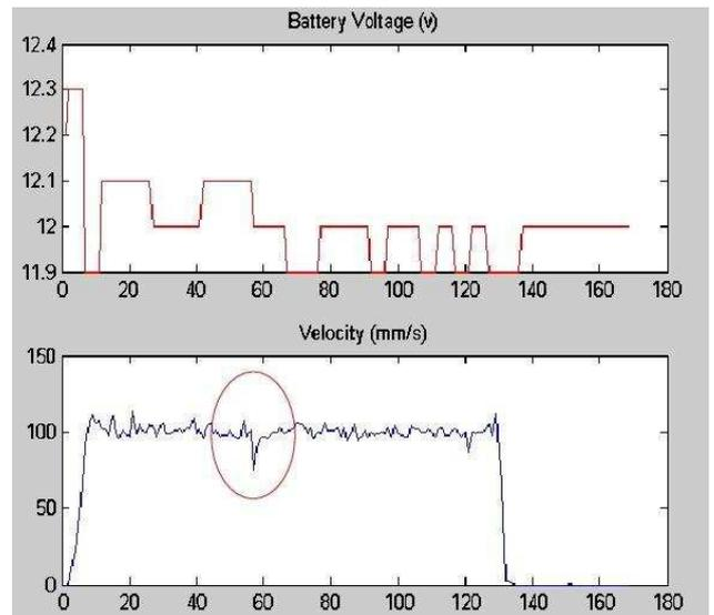
Figure 2: Vehicle Battery Voltage and Linear Velocity during a collision-and-drag case.
