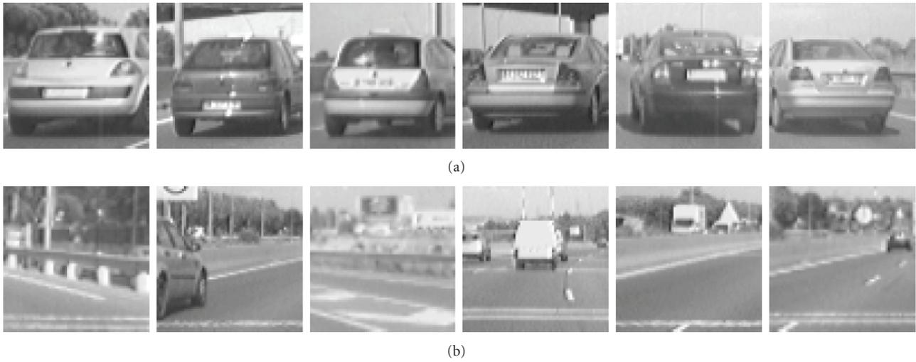
FIGURE 12: Forward data set. (a) positive samples (vehicles). (b) negative samples.
