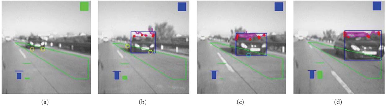
FIGURE 7: Example of the side-vehicle detection module (also called *blind spot* detection) in a sequence of images. The indicator in the upper-right part of the figure toggles from green to blue when a car is detected in the blind spot.
