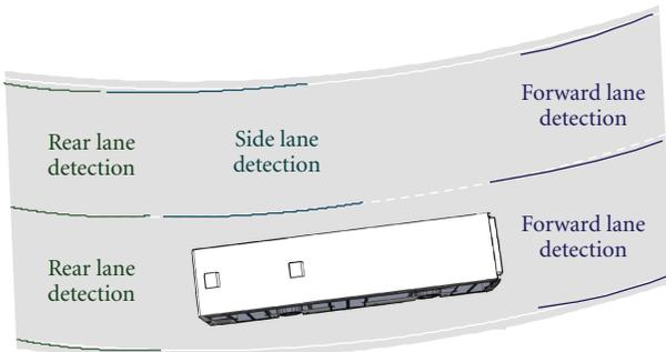
FIGURE 4: Rear, side, and forward lane detection.
