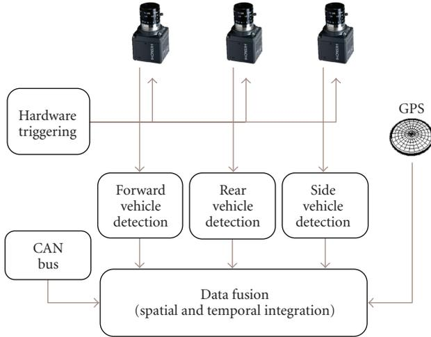
FIGURE 3: Stages of the vision-based traffic detection system.
