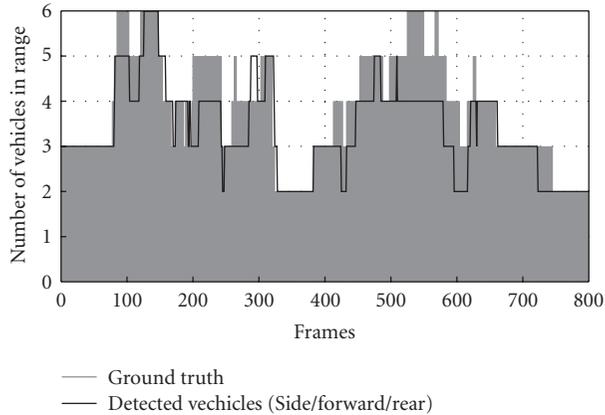
FIGURE 16: Number of vehicles detected by the three vision modules compared with the manually labeled ground truth in a real sequence.
