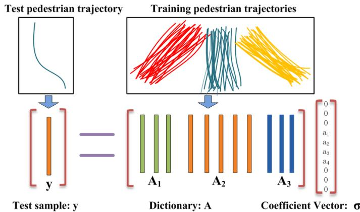
Figure 1 An example of the sparse representation technique applied in pedestrian trajectories understanding.
