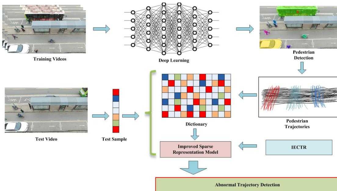
Figure 2 The preprocessing flow for pedestrian trajectory extraction and collection.
