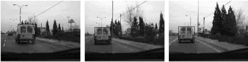
Fig. 4. Detection of a sudden braking of the preceding vehicle by continuously monitoring the activation of the braking lights.
