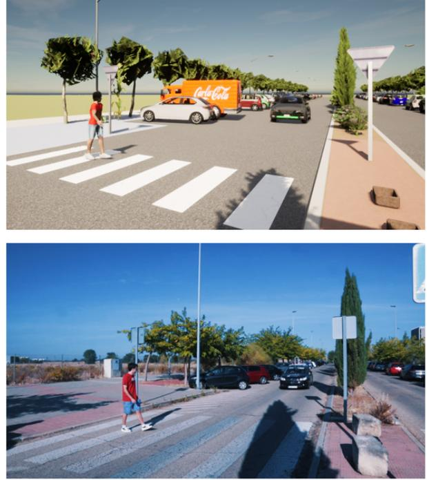
Fig. 1. Digital twin for human-vehicle interaction in autonomous driving, a comparison between virtual (above) and real (bottom) experiments.
