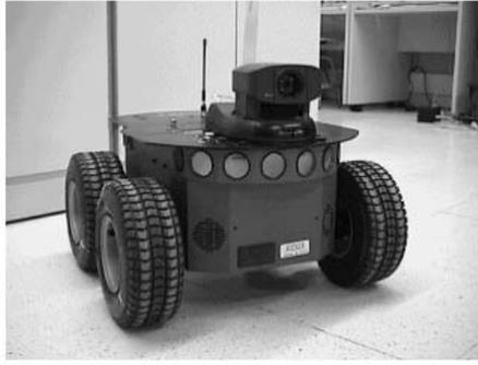
**Fig. 4.** UAH platform: BART (Basic Agent for Robotic Tasks) robot.
