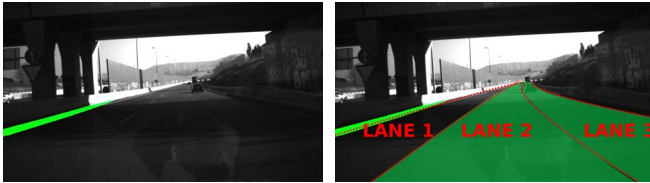
Fig. 3: Left: Only one of four lines are detected. Right: The highlighted lanes (two and three) have a higher probability of being the vehicle ego-lane, as the evaluation of the relative distance w.r.t. detected line implies.
