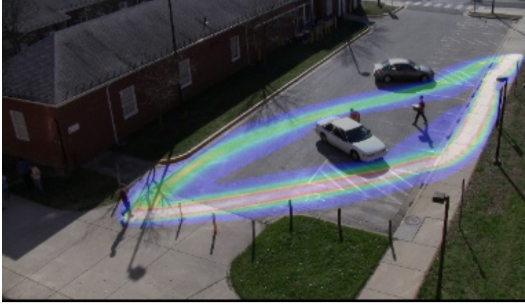
Figure 2.2: Given a single pedestrian detection, the approach proposed in [33] forecasts plausible paths and destinations from vision-input. Physical attributes of the scene are able to encode agent preferences like using the sidewalks.
