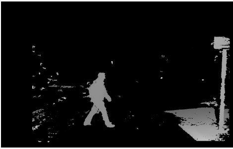
(c) Depth map where values which correspond to the ground plane were removed.
