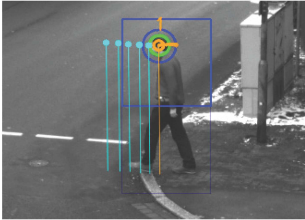
Figure 2.4: Prediction of pedestrian path during a gait initiation with an interval of 0.2 seconds computed by the algorithm described in [20].
