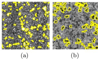
**Fig. 3.** Maximally stable extremal regions detection. a) white blobs. b) black blobs.
