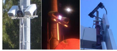
Fig. 8. Different stereo platforms with IR illuminator.
