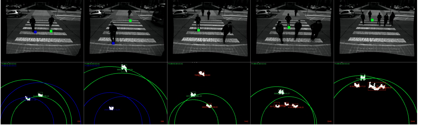
Fig. 4. Upper row: left image with color-coded identification. Lower row: XZ-map (top-view without road points), detected blobs and RSSI circumferences. Each tag is labeled with a different color.
