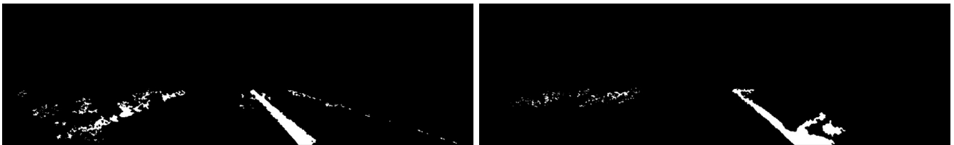
(d) Output of the curb detection algorithm for the stereo point cloud
