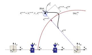
Fig. 6. Example of the proposed distance metric between a blob and a tag for the right antenna.
