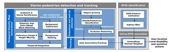
Fig. 2. Flowchart representation of the overall approach.
