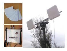
Fig. 9. Left: RFID TAGs and reader; Right: platform with RFID antennas and cameras.
