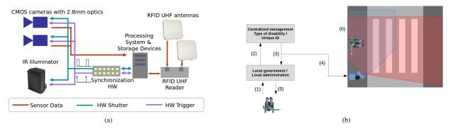
Fig. 1. (a) Sensor architecture; (b) General procedure for anonymous identification.
