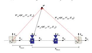
Fig. 4. Relative position between cameras and RFID antennas.
